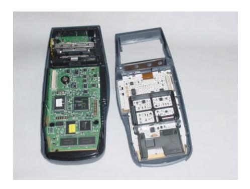
**EUT – Back View of Mother PCB and Front of Radio**
