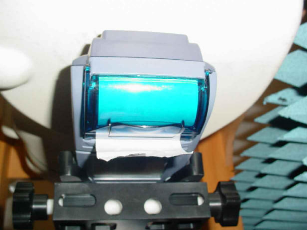
Photo 10: Test position body worn rear side (10 mm distance)
