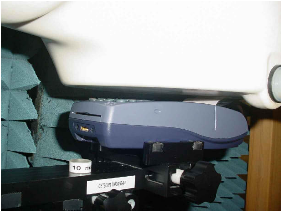
Photo 8: Test position body worn front side (10 mm distance)
