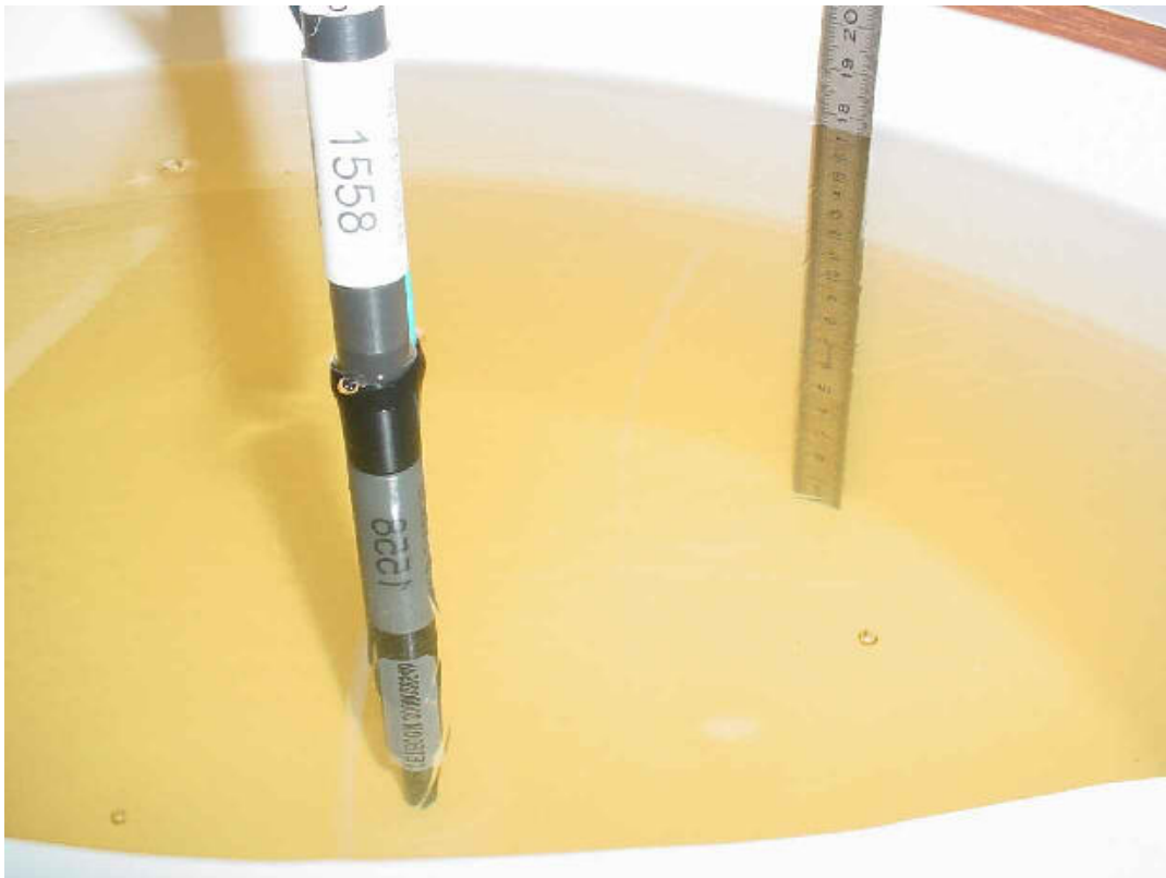
Photo 12: Liquid depth 1900 MHz body simulating liquid
