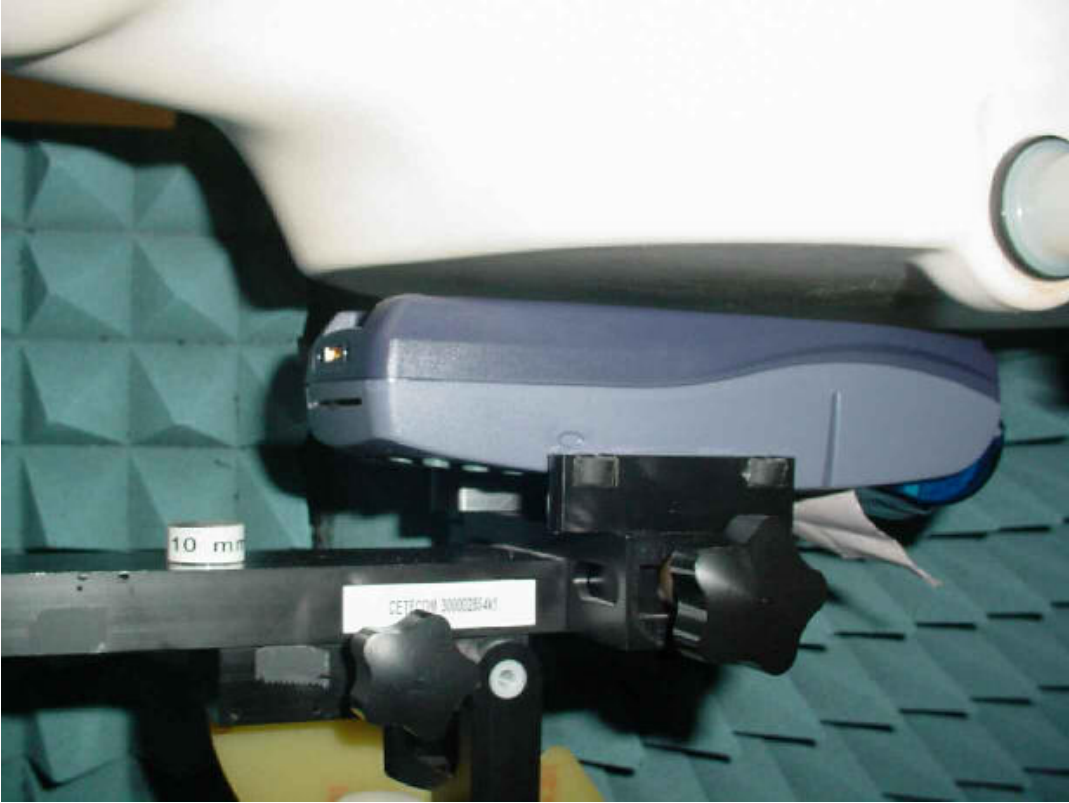
Photo 10: Test position body worn rear side (10 mm distance)
