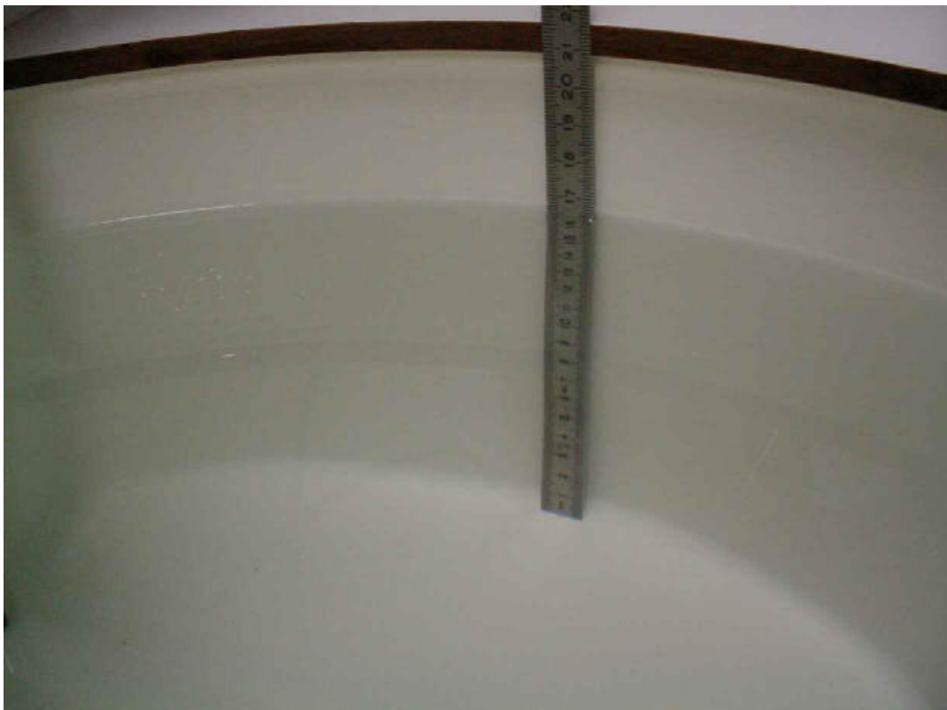
Photo 12: Liquid depth 1900 MHz body simulating liquid
