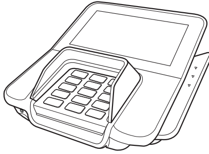
Figure 22 Privacy Shield attached to Terminal
