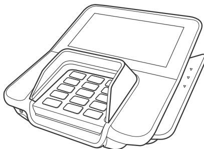
Figure 15 Privacy Shield attached to Terminal
