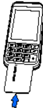
Figure 3 Inserting a Smart Card
