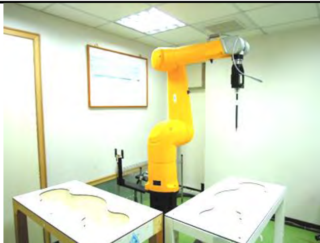
Fig-3.2 SPEAG DASY52 System
