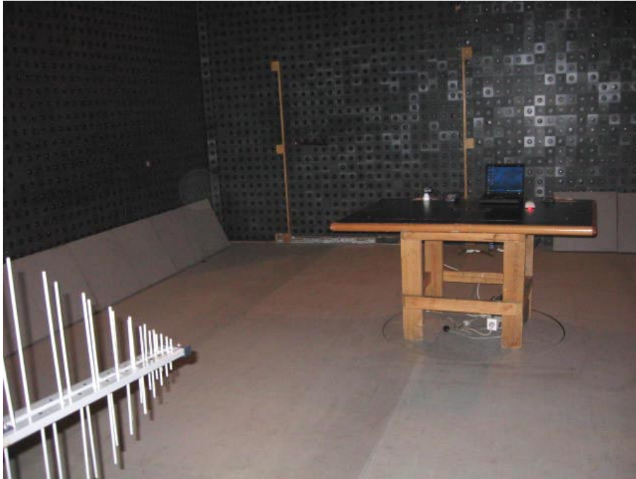
Photograph No.2 Radiated emissions measurement setup in the anechoic chamber with biconilog antenna
