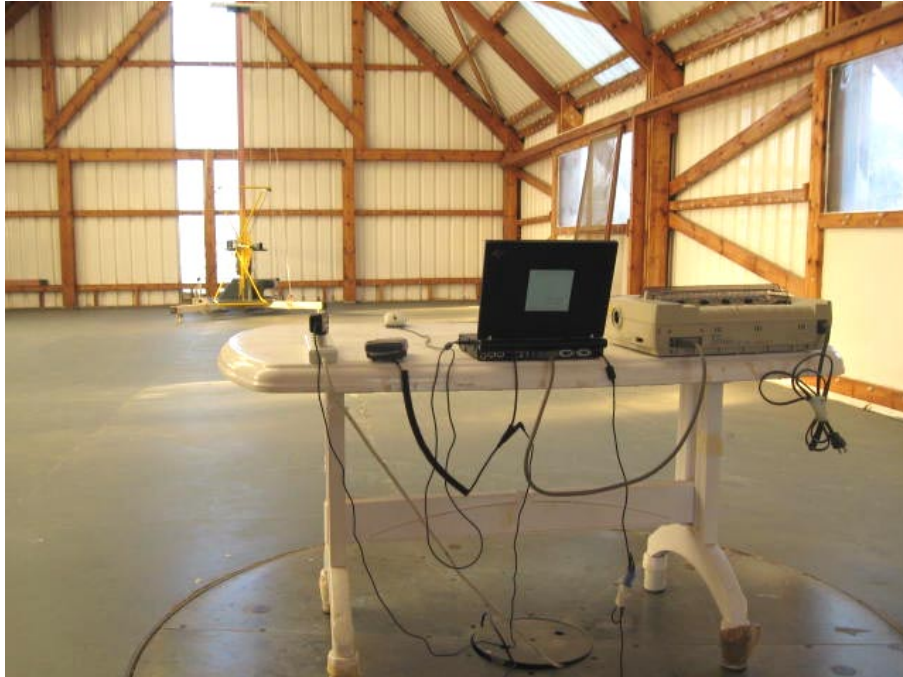
Photograph No.3 Radiated emissions measurement setup at the OATS, close view
