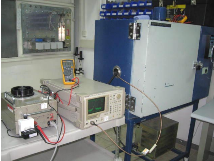
Photograph No.4 Frequency stability measurement setup
