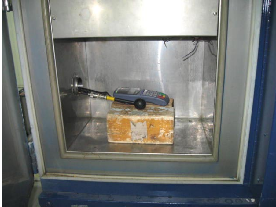
Photograph No.5 Frequency stability measurement setup
