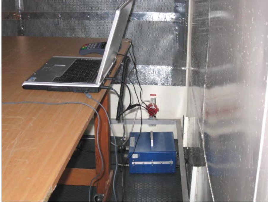
Photograph No.7 Conducted emissions measurement setup
