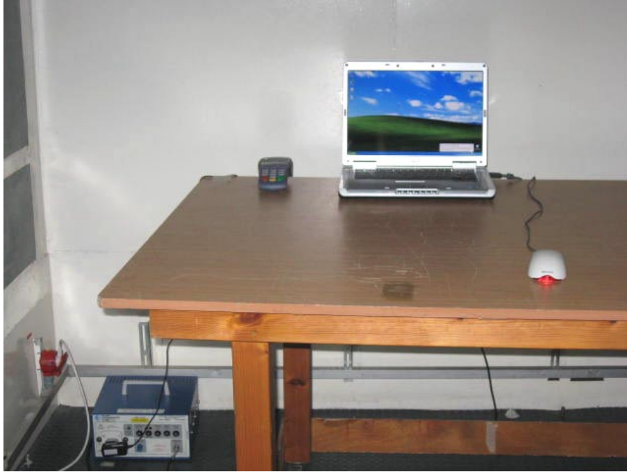
Photograph No.6 Conducted emissions measurement setup
