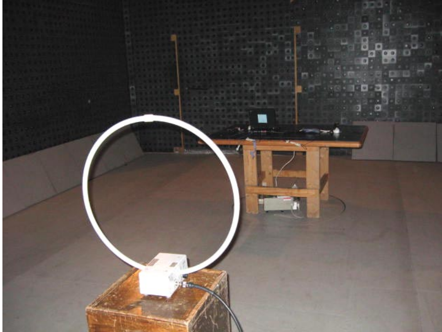
Photograph No.1 In-band and out of band radiated emissions measurement setup in the anechoic chamber with loop antenna
