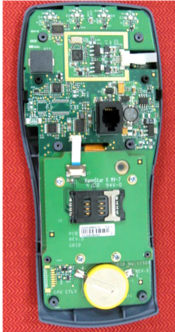
Photograph No. 1 PINpad 1000se CTLS / Qx1000 payment terminal internal view with rear panel removed
