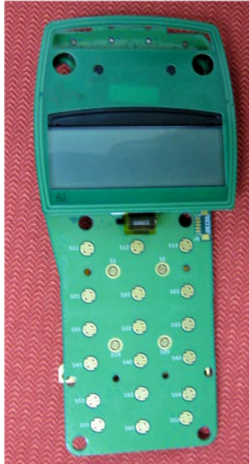
Photograph No. 4 PINpad 1000se CTL5 / Qx1000 main PCB front view with loop antenna PCB
