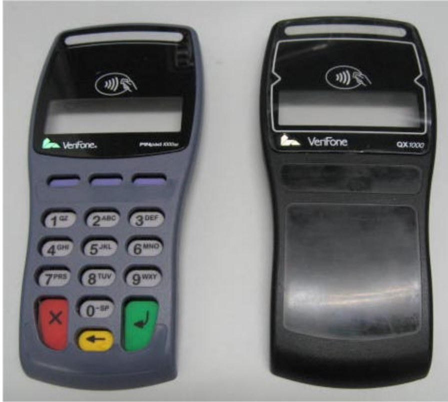
Photograph No. 3 PINpad 1000se and Qx1000 front panels
