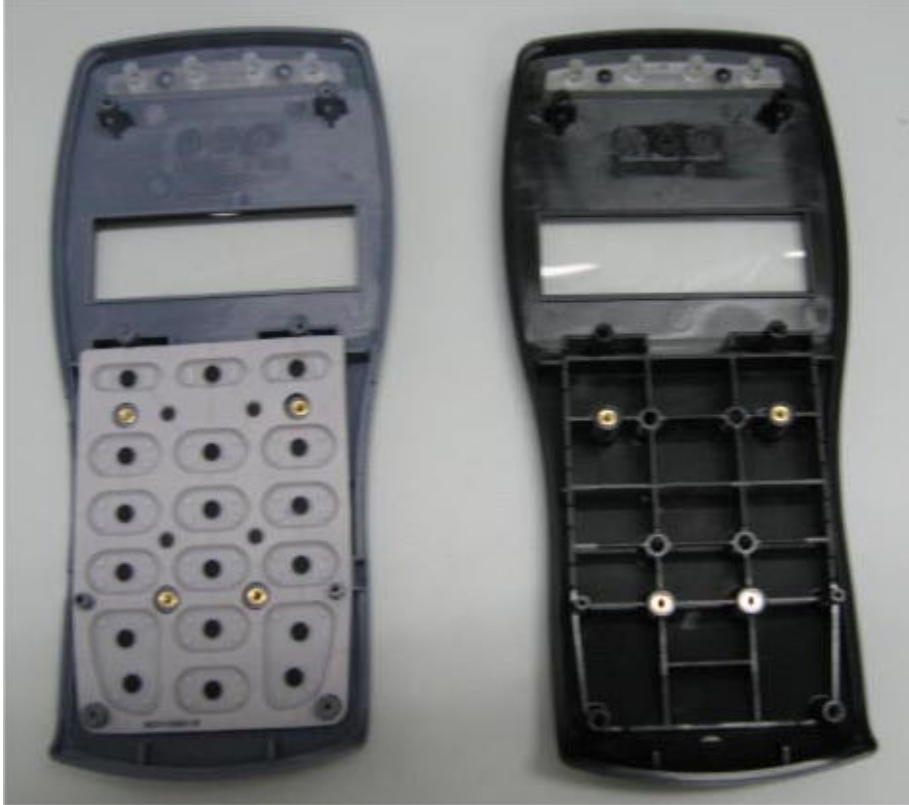
Photograph No. 4 PINpad 1000se and Qx1000 front panels inside view
