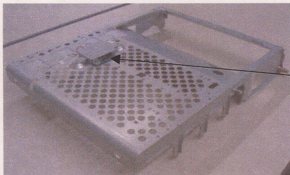
Shielded RF Module with case (Photo 1)
