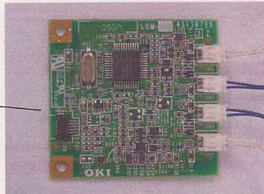
RF Module without shielding (Photo 2)
