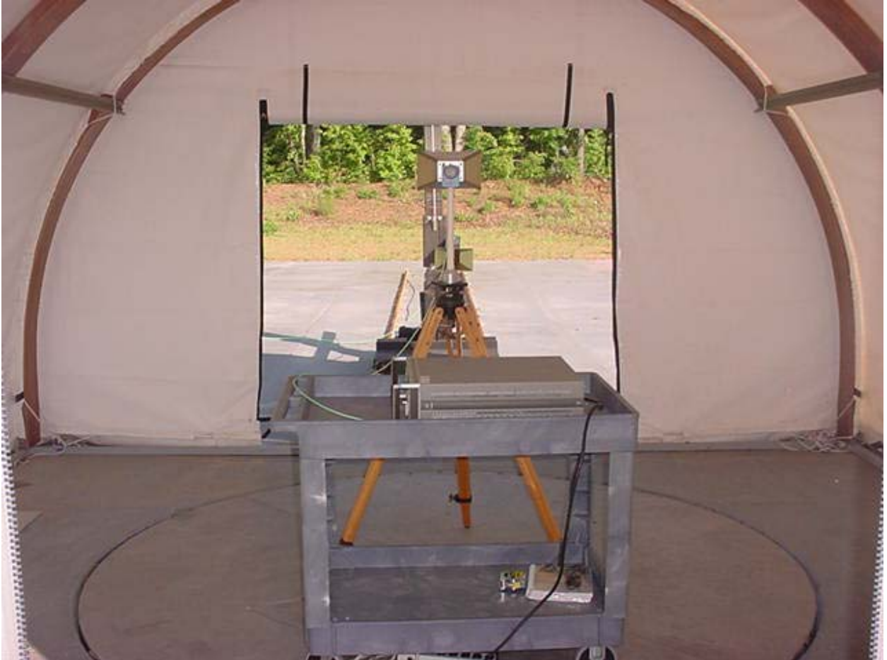
Figure 6: Substitution Field Strength – Rear View
