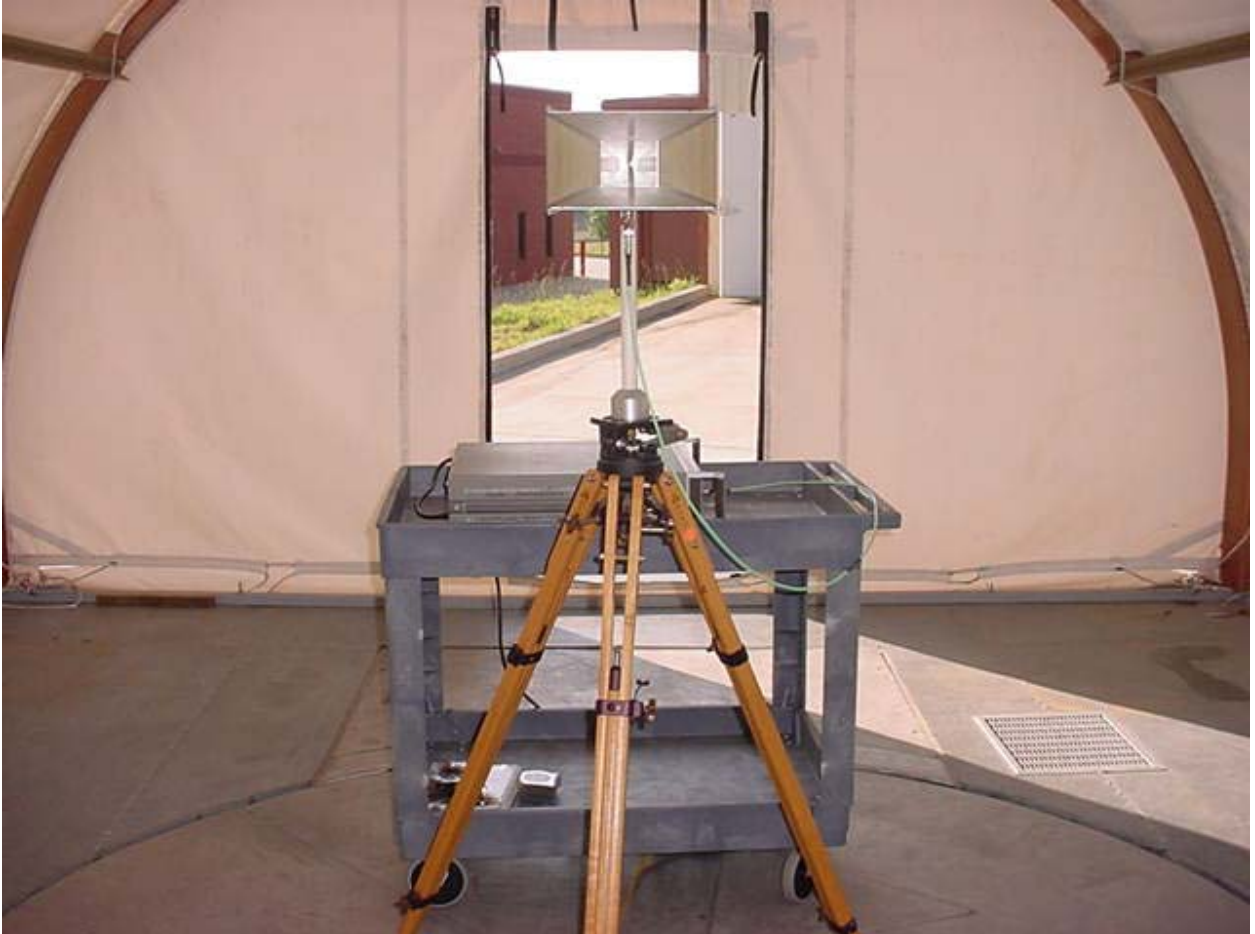
Figure 5: Substitution Field Strength – Front View
