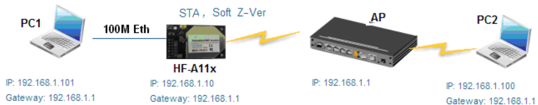
Figure 21. HF-A11x Ethernet Interface Networking (As STA, Z-Ver)
