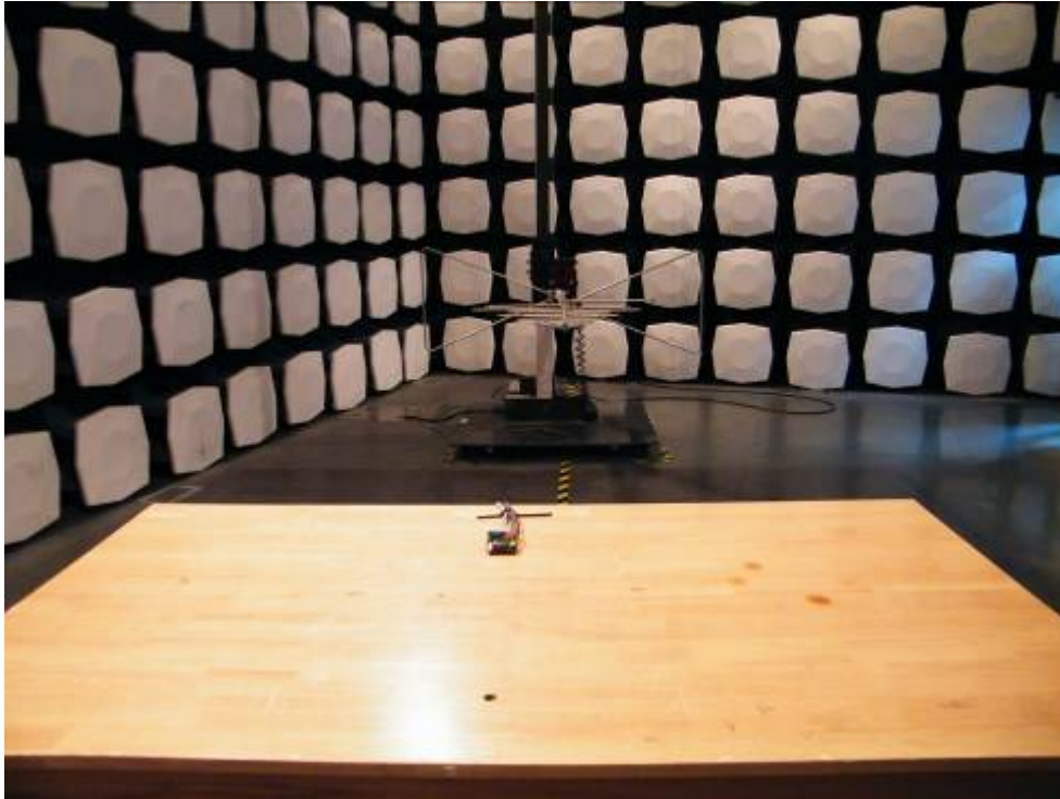
Picture 2 Radiated Emission Test Setup
