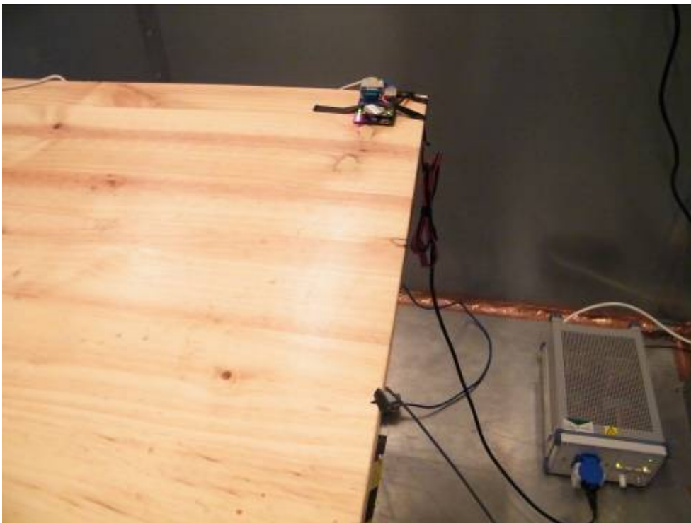
Picture 3 Conducted Emission Test Setup
