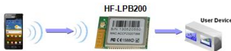
Figure 32. Wireless Control Application
