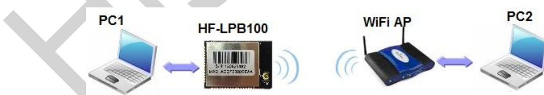
Figure 23. STA Interface Debug Connection
