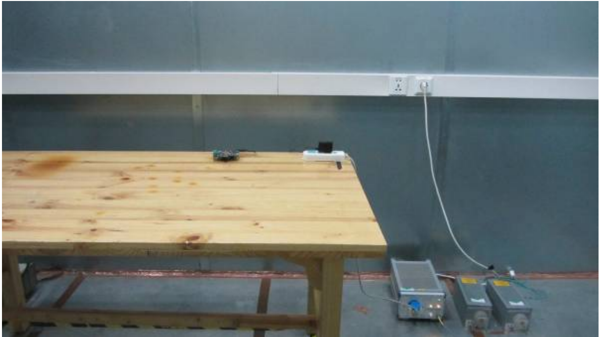
Picture 3 Conducted Emission Test Setup
