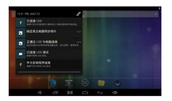
Press "USB connected", select "Turn on USB storage". The device is recognized at Explorer of the computer. Now you can use it as an external storage.
