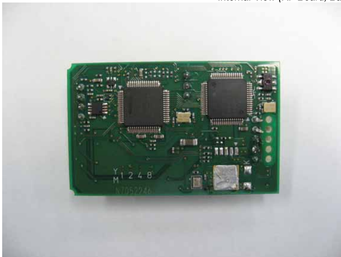
Figure 11 Internal View (RF Board, Back View)
