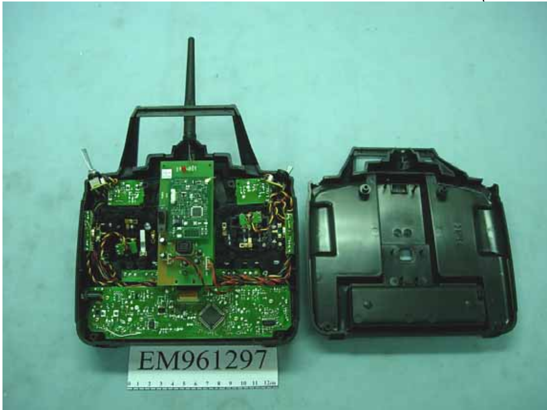
Figure 8 Internal View (Removed Cover)
