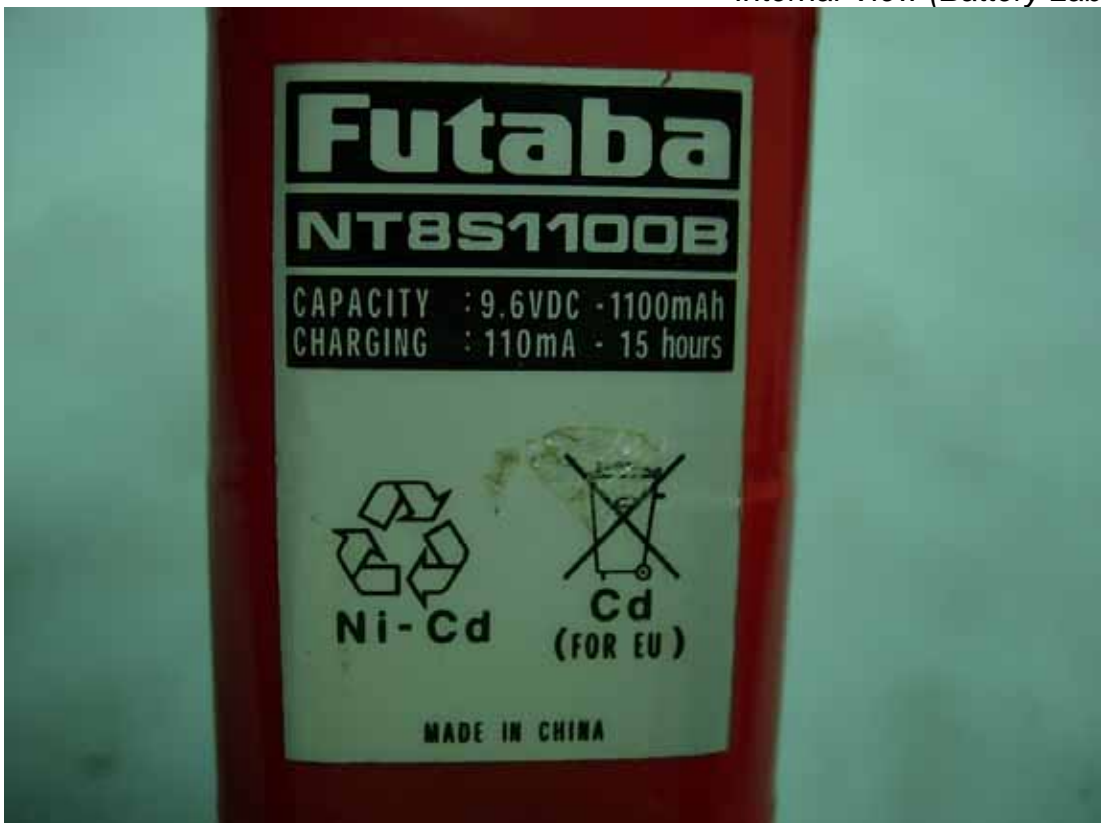
Figure 7 Internal View (Battery Label View)
