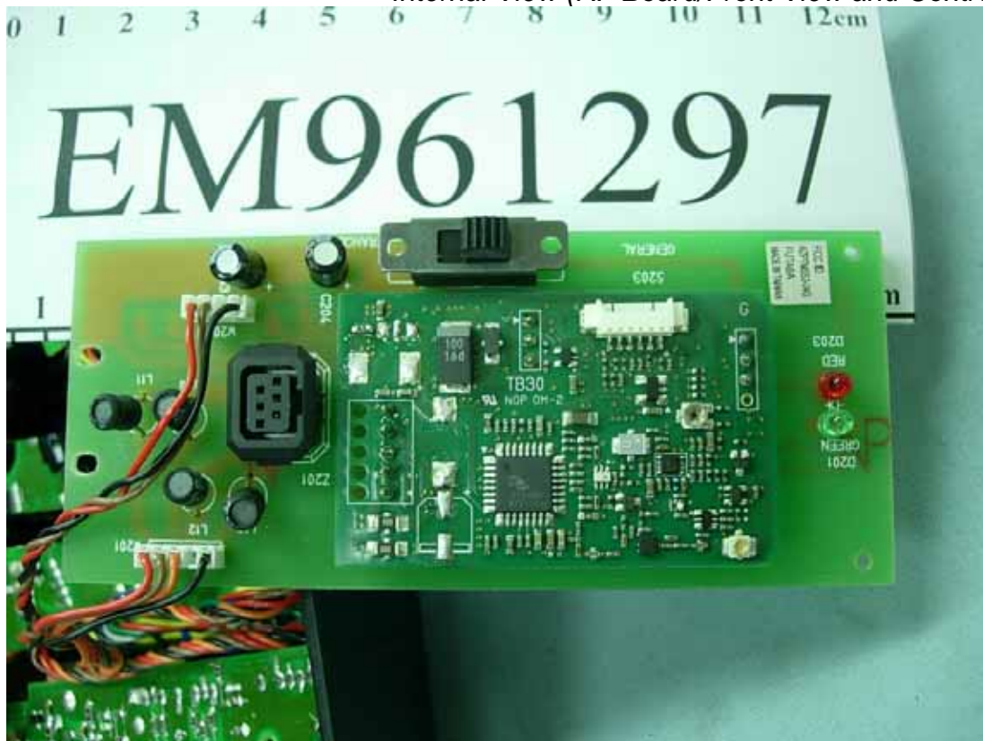
Figure 10 Internal View (RF Board/Front View and Control Board)
