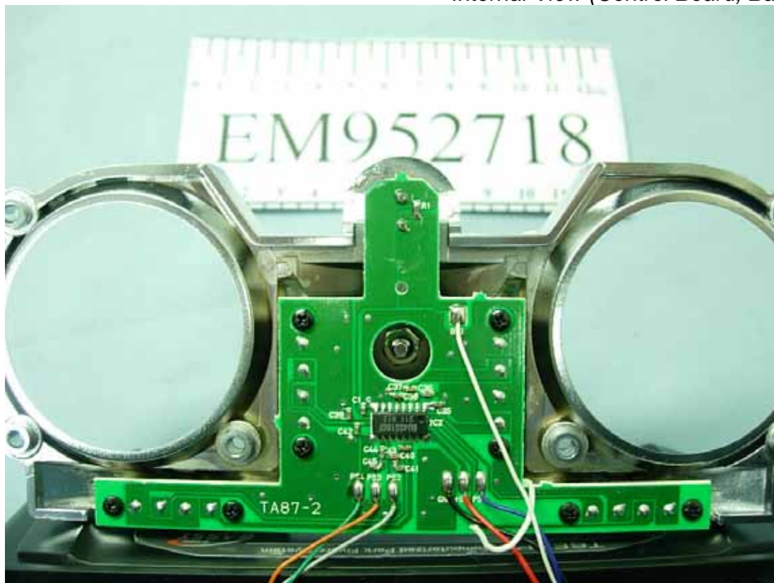
Figure 17 Internal View (Control Board, Back View)
