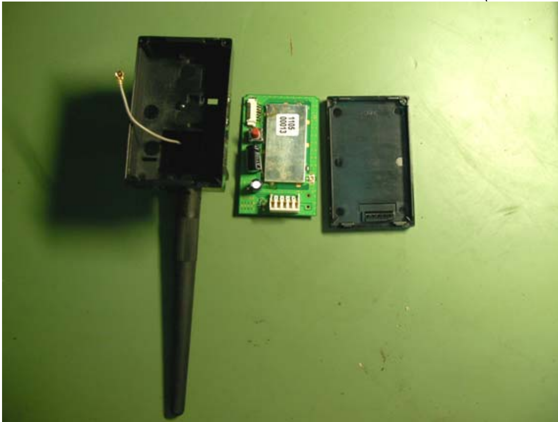
Figure 3 Internal View (Removed Covers)
