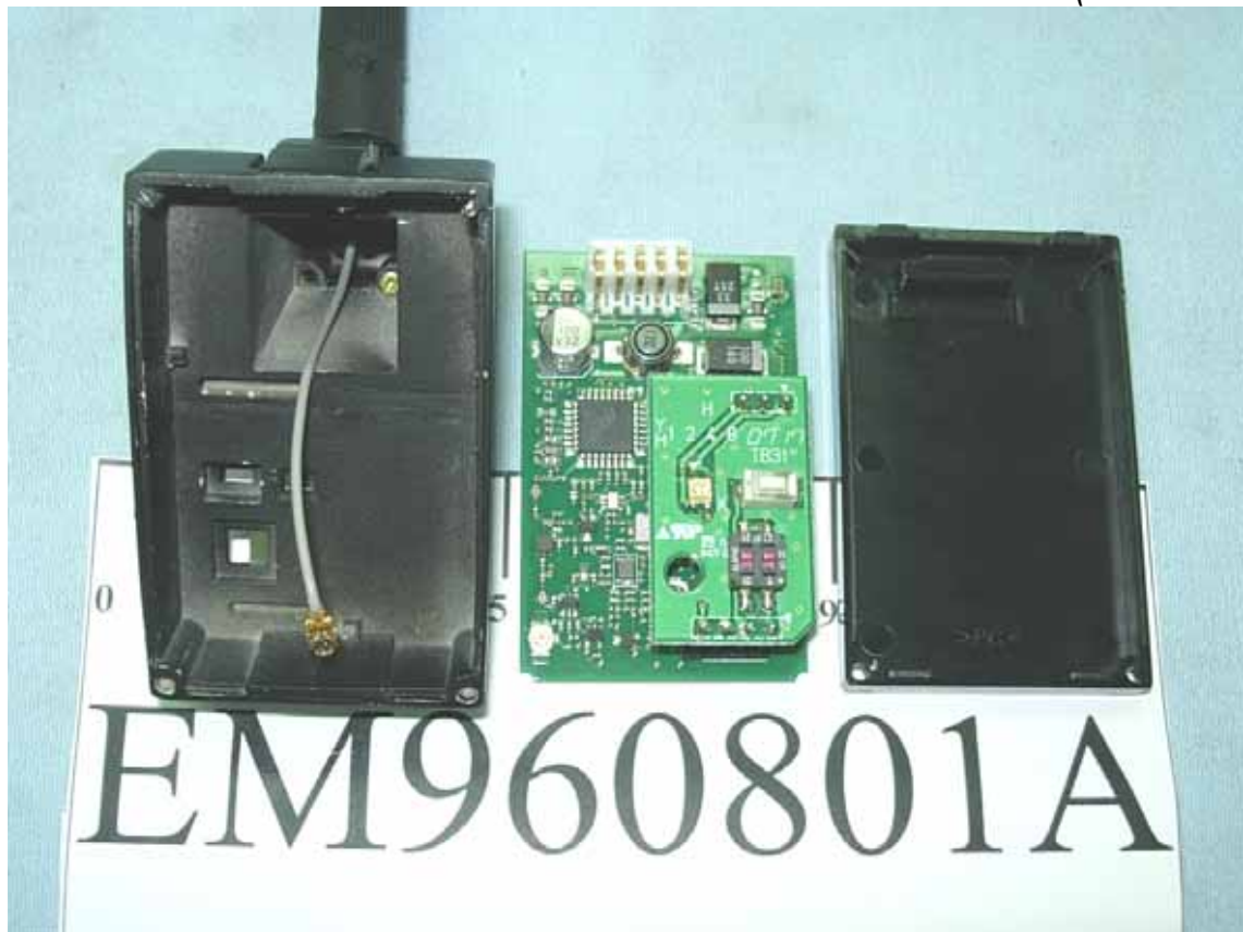
Figure 5 Internal View (Cover Removed)
