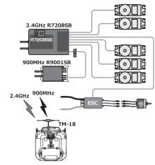
By using Futaba AdRCSS 900MHz and Futaba 2.4GHz system together will provide the better secure RF link.
