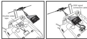
\* In the case of T32MZ, attach the included mounting parts and double-sided tape as shown in the figure.
