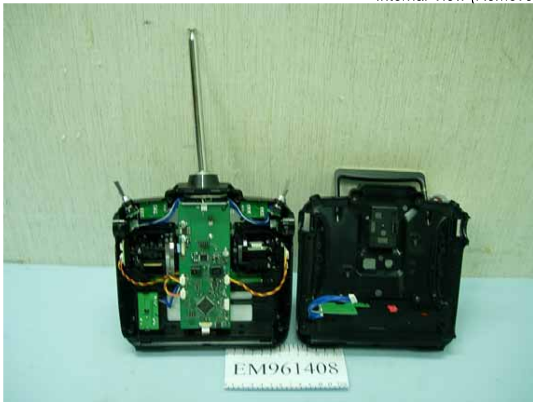
Figure 13 Internal View (Removed Cover)
