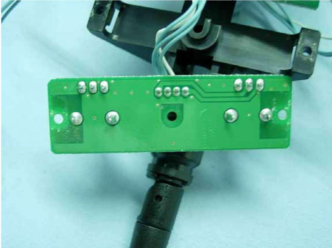
Figure 24 Internal View (Control Board, Back View)
