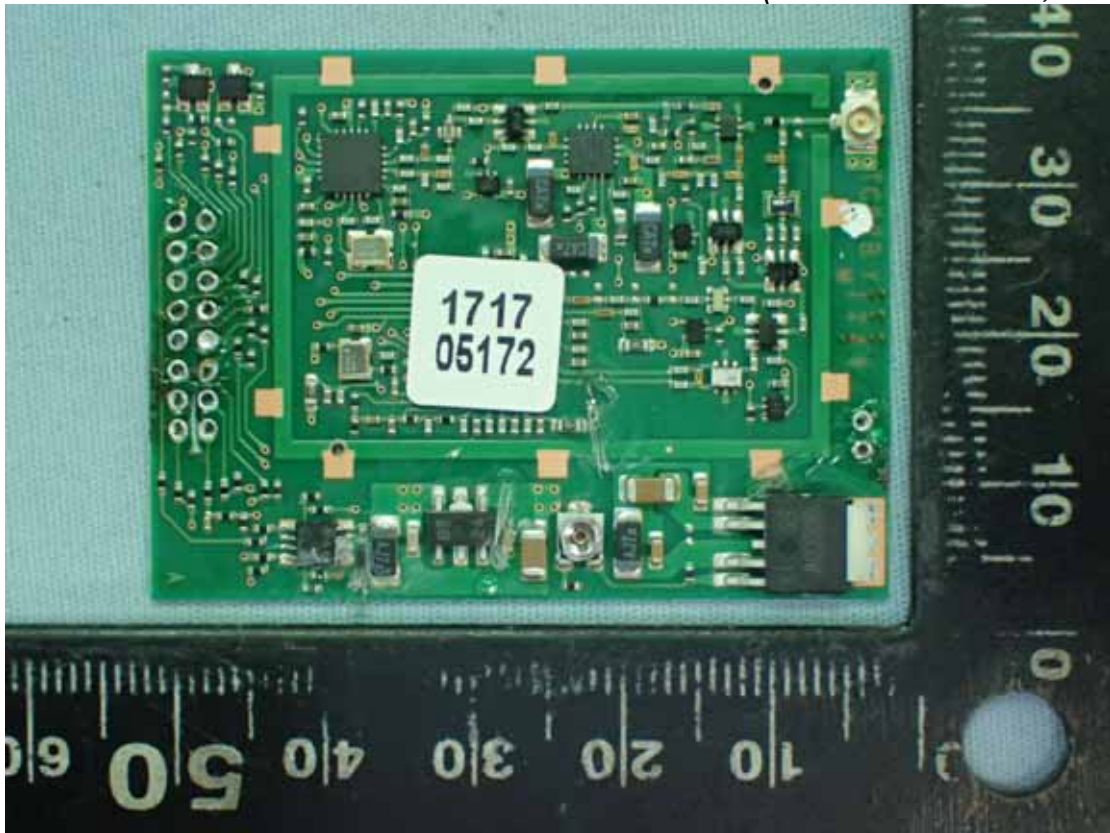
Figure 44 Internal View (RF Control Board, Front View)
