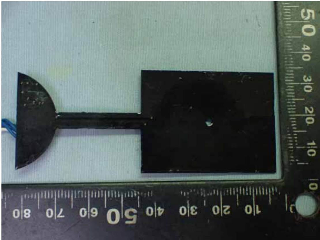
Figure 18 Internal View (NFC Antenna, Back View)
