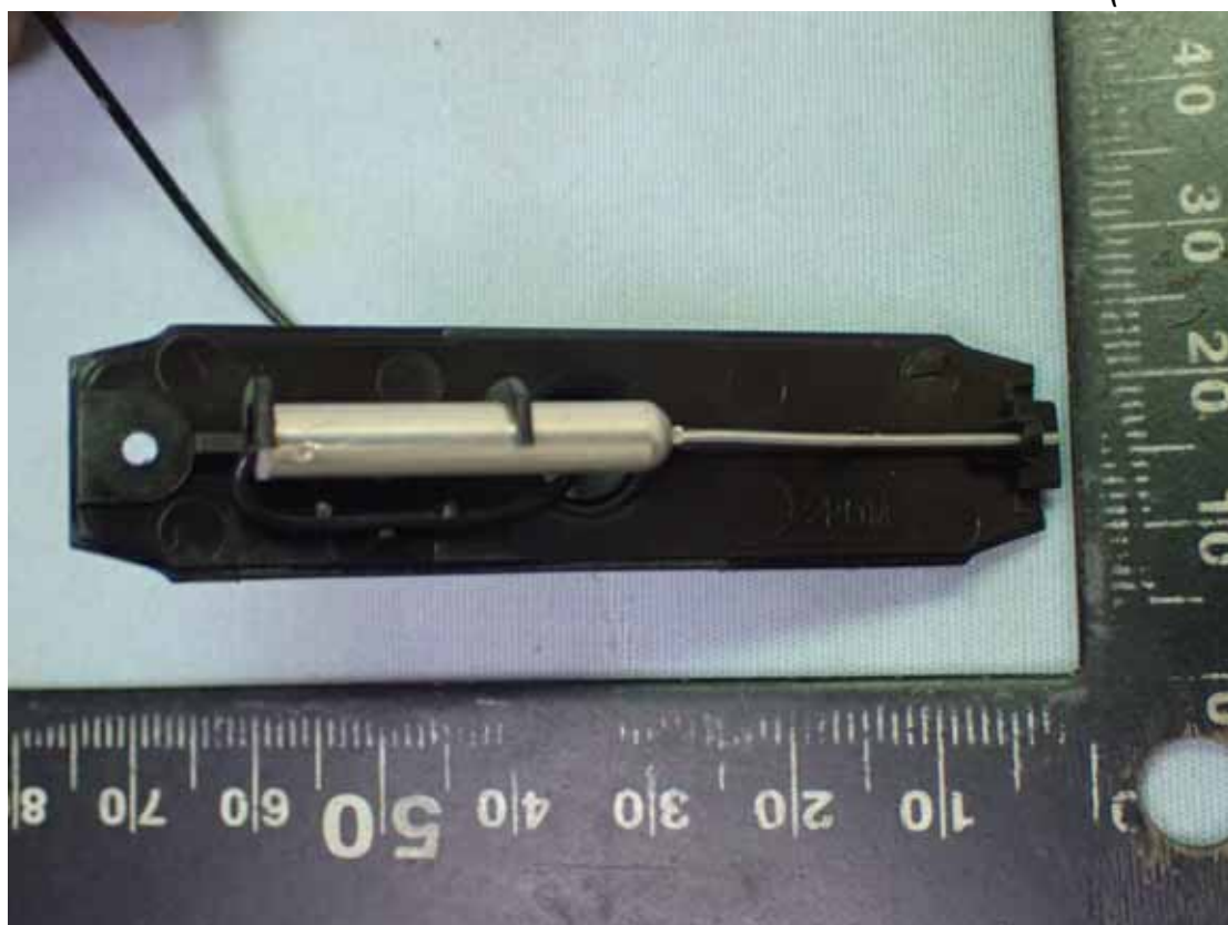
Figure 21 Internal View (Antenna View)
