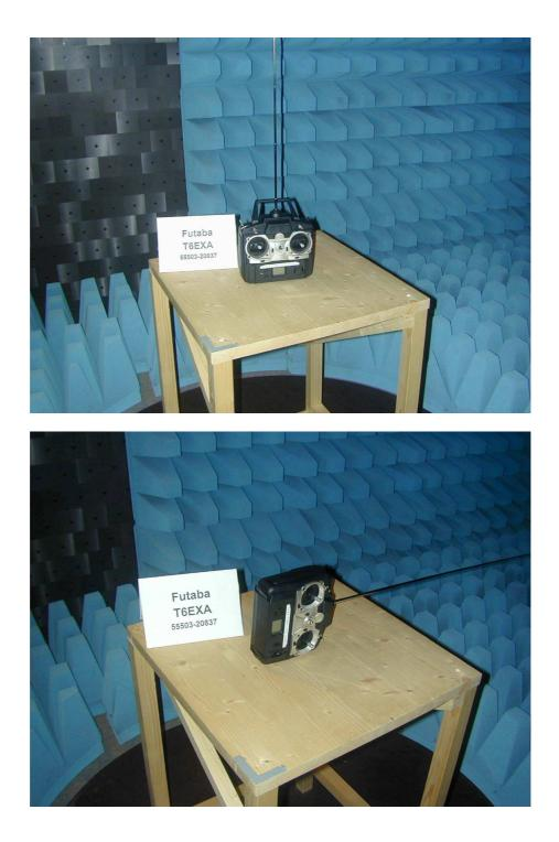
Test setup unwanted radiation 30 MHz - 1 GHz
