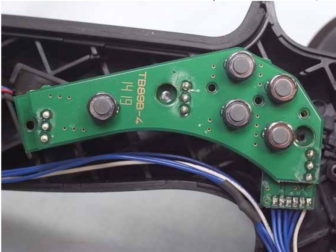
Figure 12 Internal View (Function Control Board, Front View)
