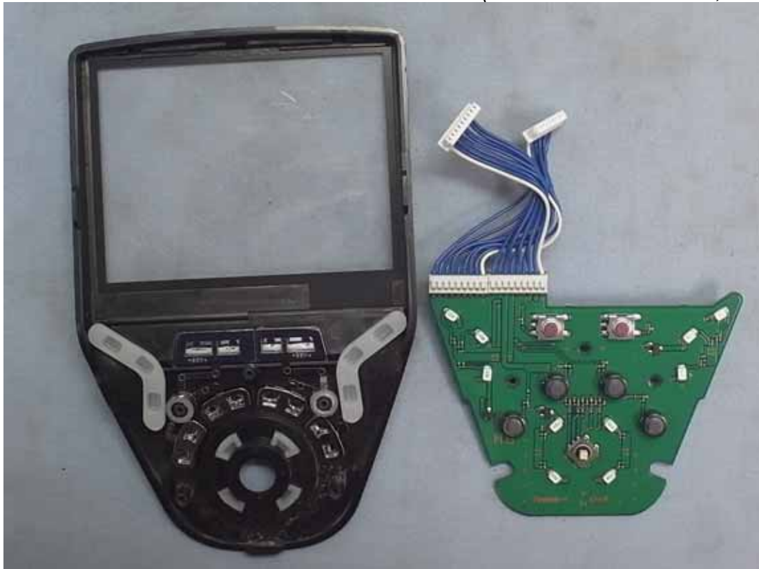
Figure 20 Internal View (Function Control Board, Front View)
