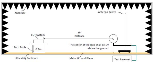
6.1.3. Setup Diagram for 30-1000 MHz
