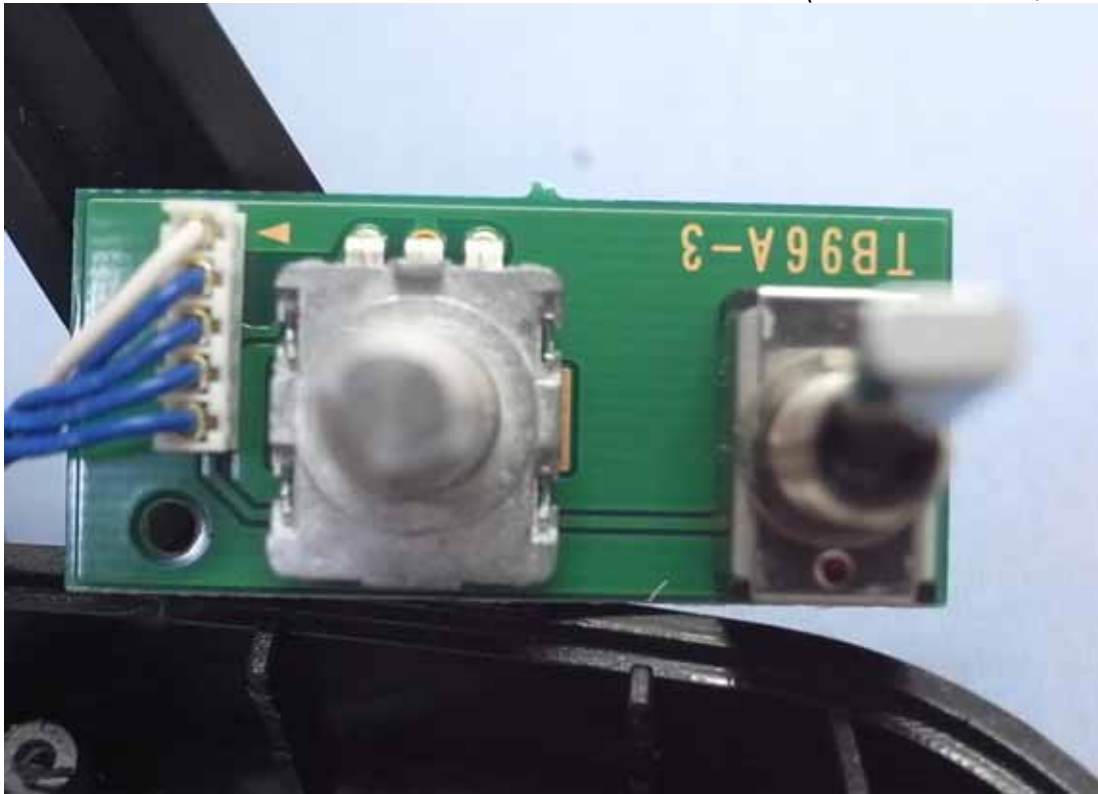
Figure 15 Internal View (TB96A-3 Board, Front View)
