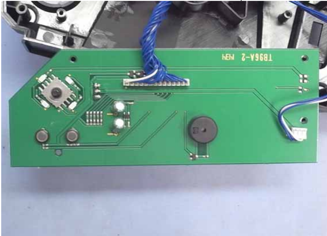
Figure 13 Internal View (TB96A-2 Board, Front View)
