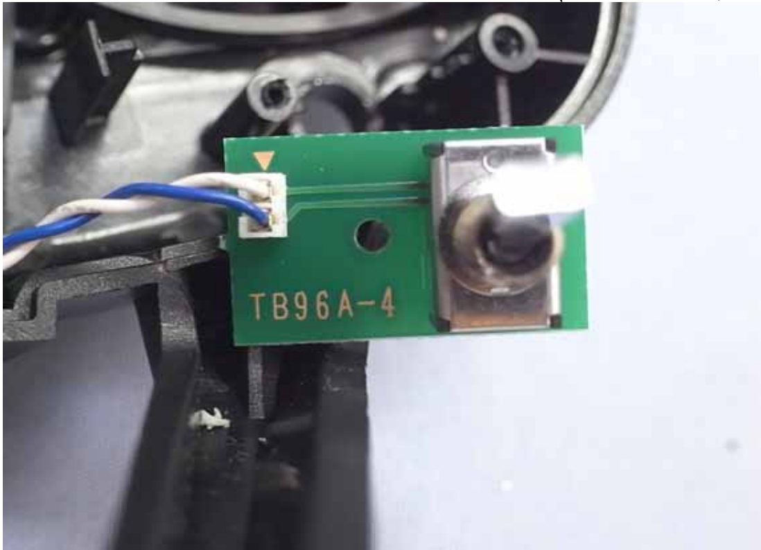
Figure 17 Internal View (TB96A-4 Board, Front View)
