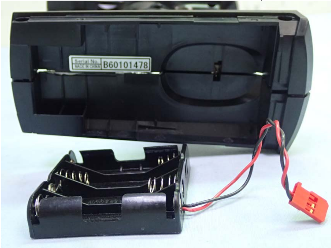
Figure 6 Internal View (Removed Battery Case)
