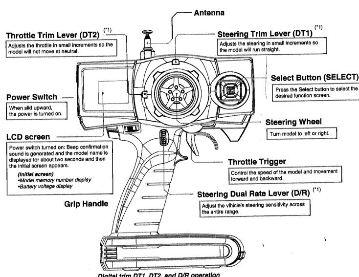
Digital trim DT1, DT2, and D/R operation Push the lever to the left or right (up or down).
