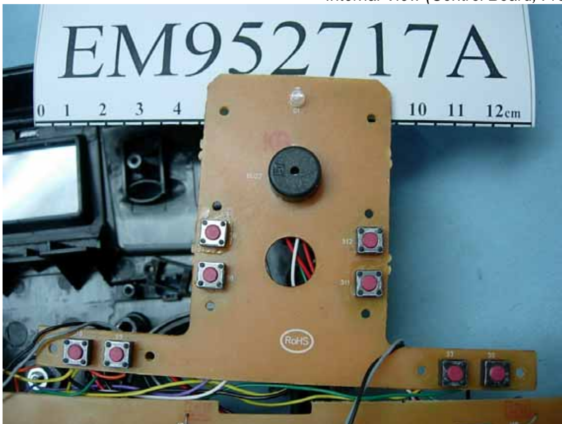
Figure 17 Internal View (Control Board, Front View)
