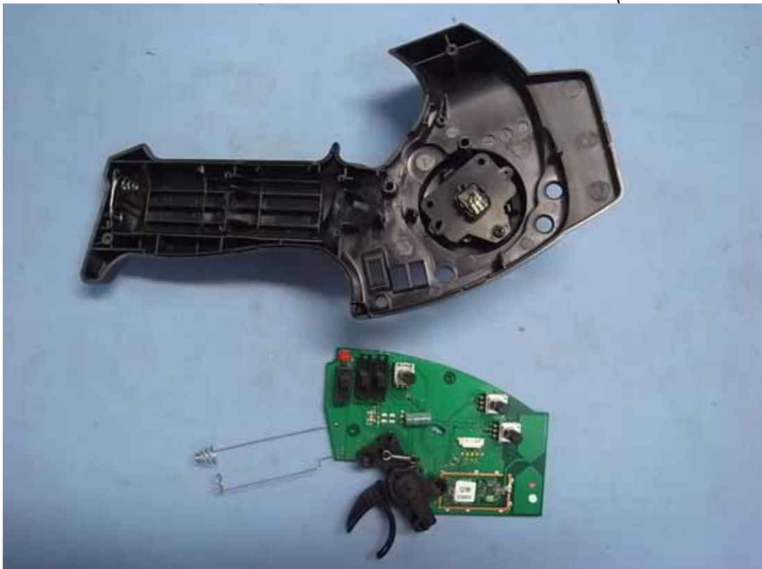
Figure 6 Internal View (Removed Main Board)
