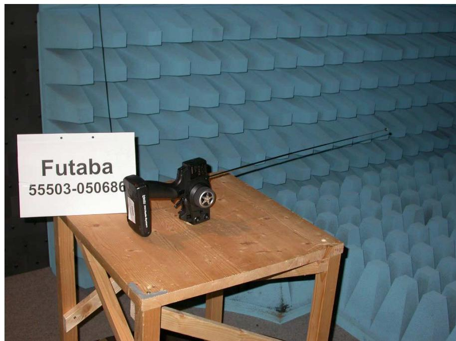
**Test setup for carrier frequency stability measurement**
