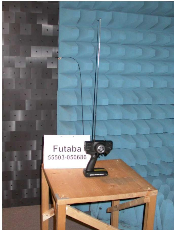
**Test setup for radiated emission measurement
