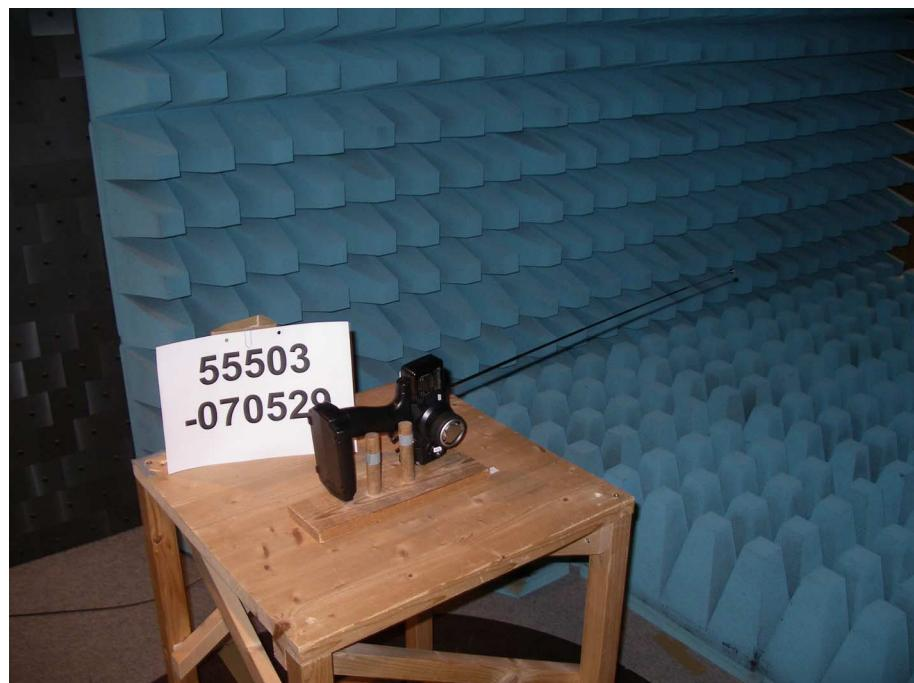
**Test setup for radiated emission measurement
