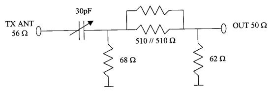
Attached RF Load provides 20dB attenuation.
