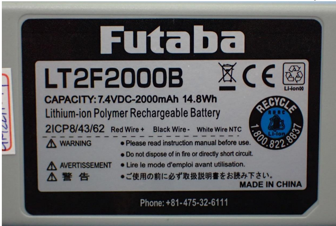
Figure 18 Battery, Label View
