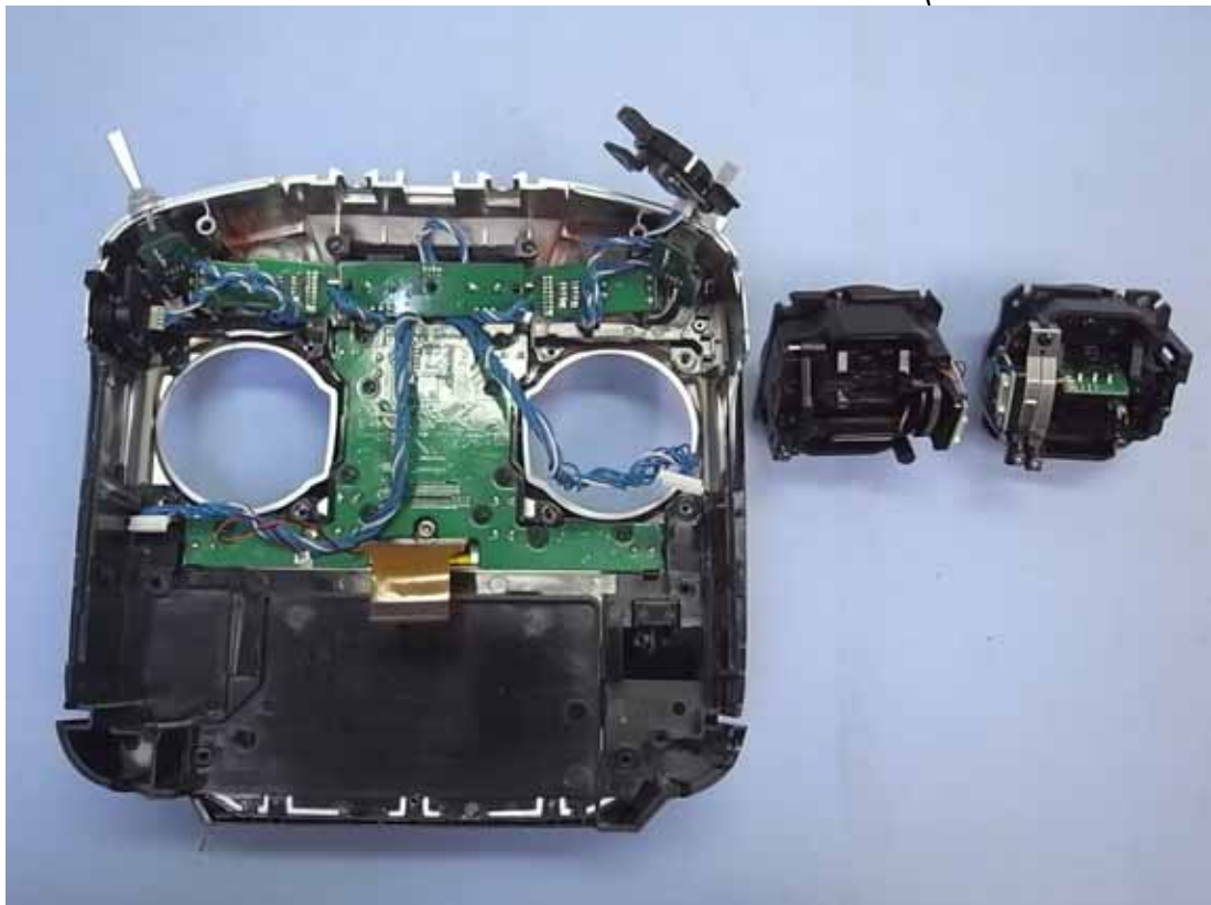
Figure 12 Internal View (Removed Control Boards)
