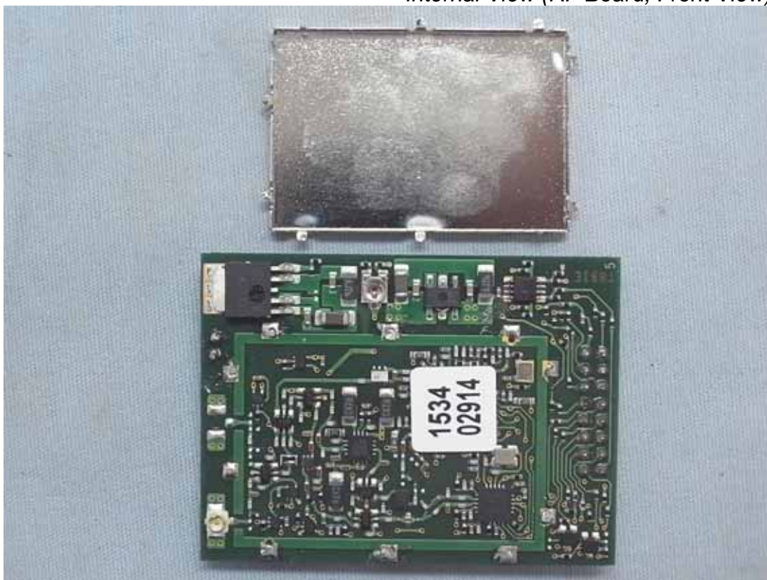
Figure 25 Internal View (RF Board, Front View)
