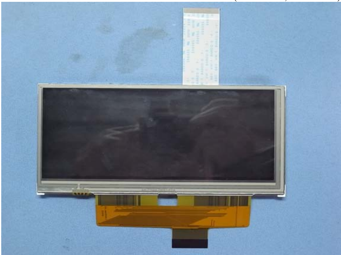
Figure 50 Internal View (LCD Panel, Back View)
