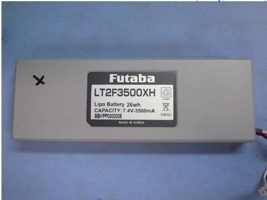
Figure 9 Internal View (Battery, Front View)
