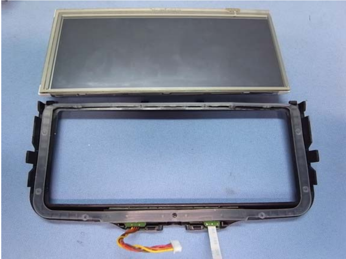
Figure 45 Internal View (LCD Panel, Removed Front Frame)
