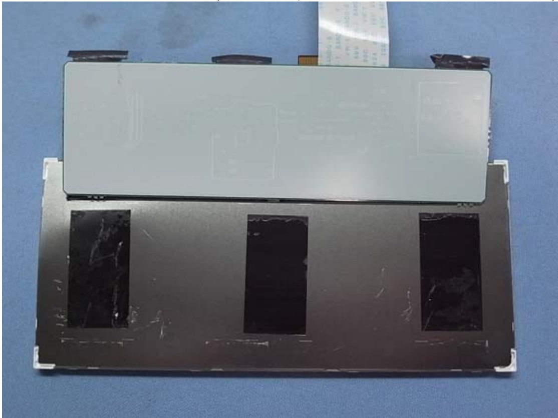
Figure 49 Internal View (LCD Panel, Removed LVDS Board/Back View)
