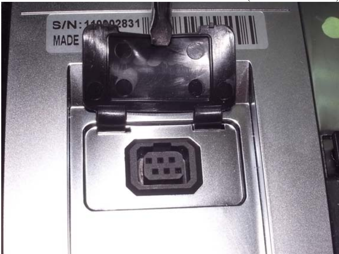
Figure 14 Internal View (Removed I/O Cover)
