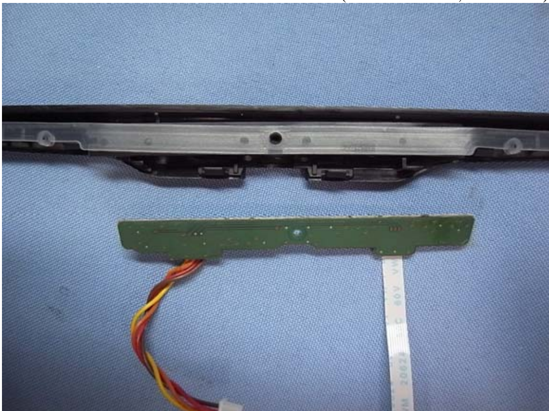
Figure 46 Internal View (TB55D-7 Board, Back View)
