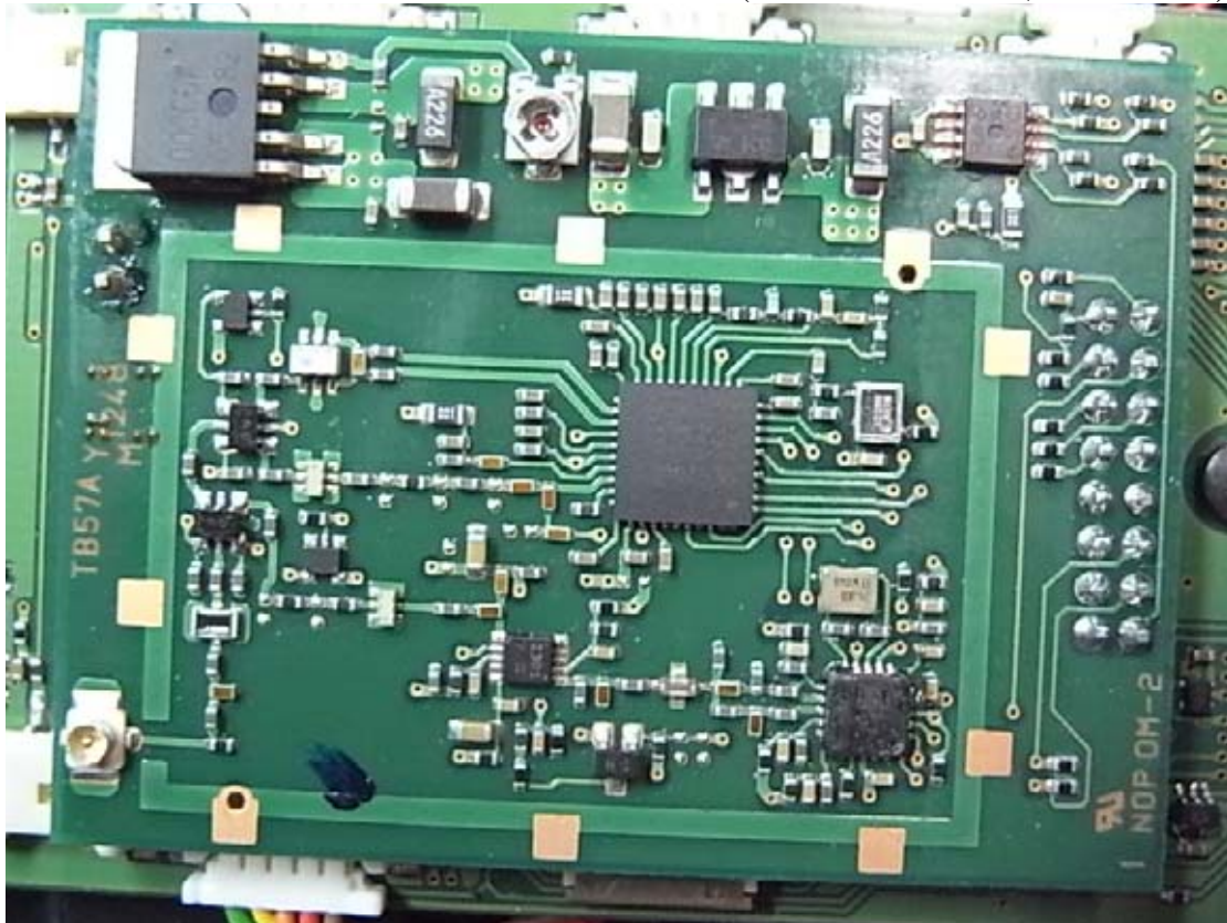
Figure 25 Internal View (TB57A RF Board, Back View)
