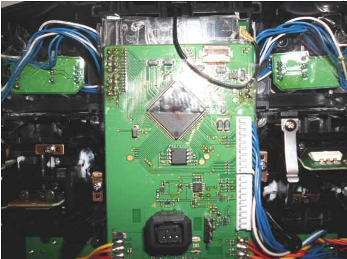
Figure 10 Internal View (RF Antenna View)
