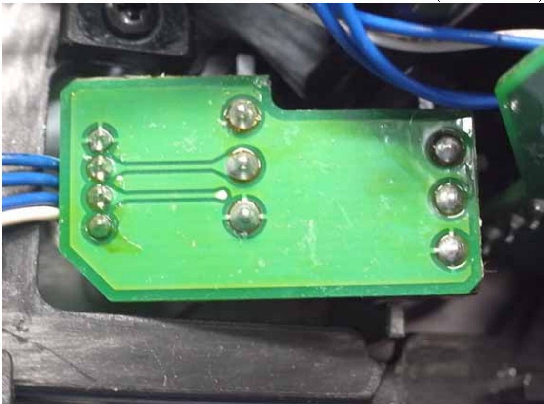
Figure 16 Internal View (Control Board)
