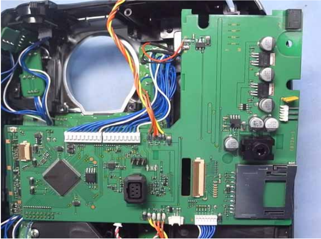
Figure 25 Internal View (TB72A-1 Board, Front View)
