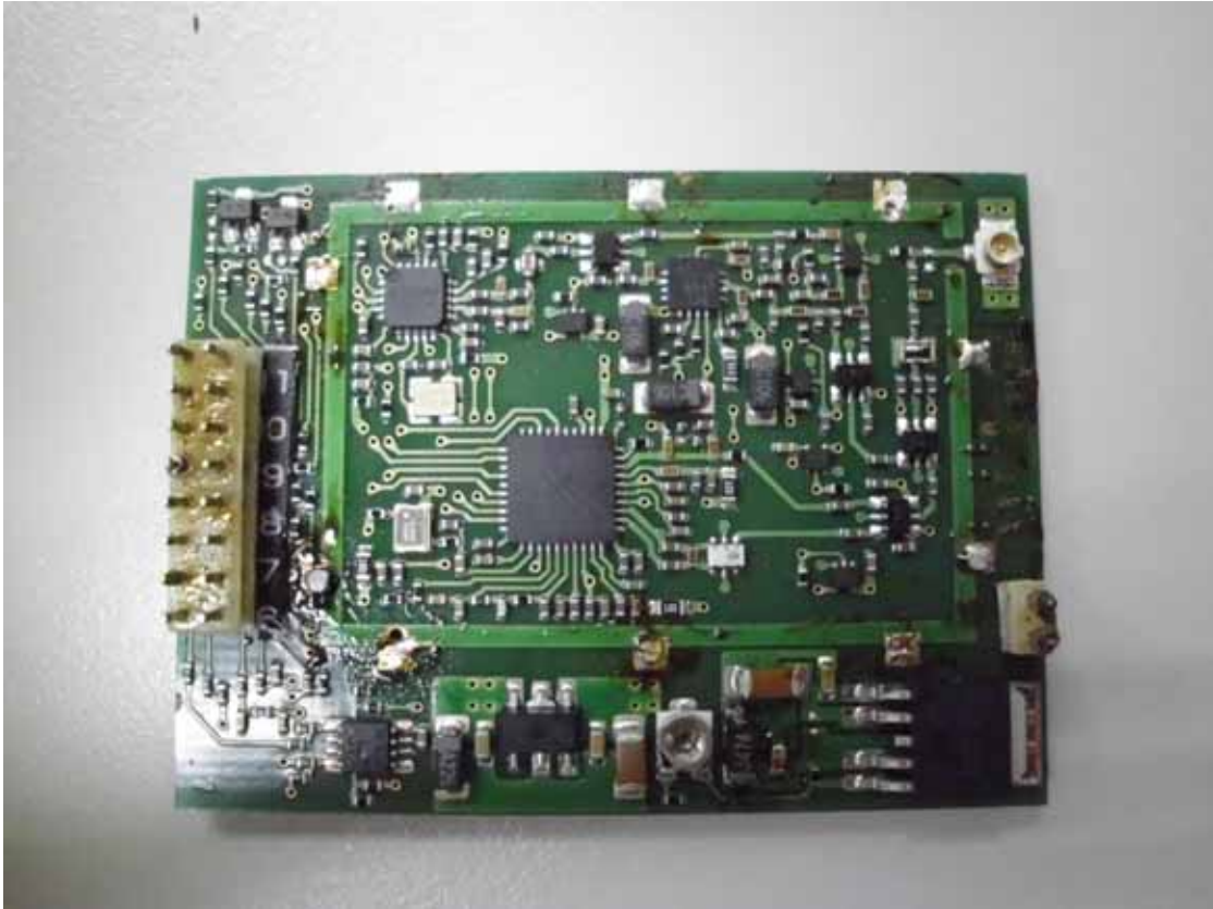
Figure 23 Internal View (RF Module Board/Removed shielded Cover, Front View)
