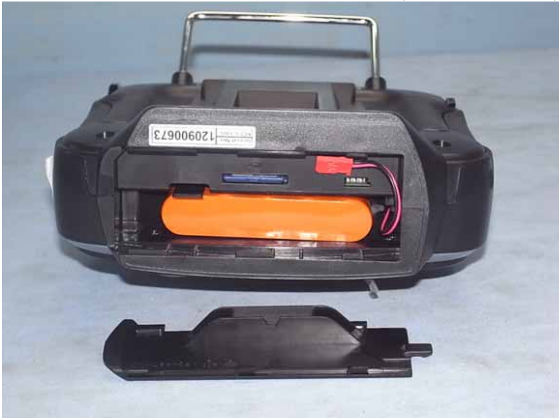
Figure 6 Internal View (Battery, Front View)
