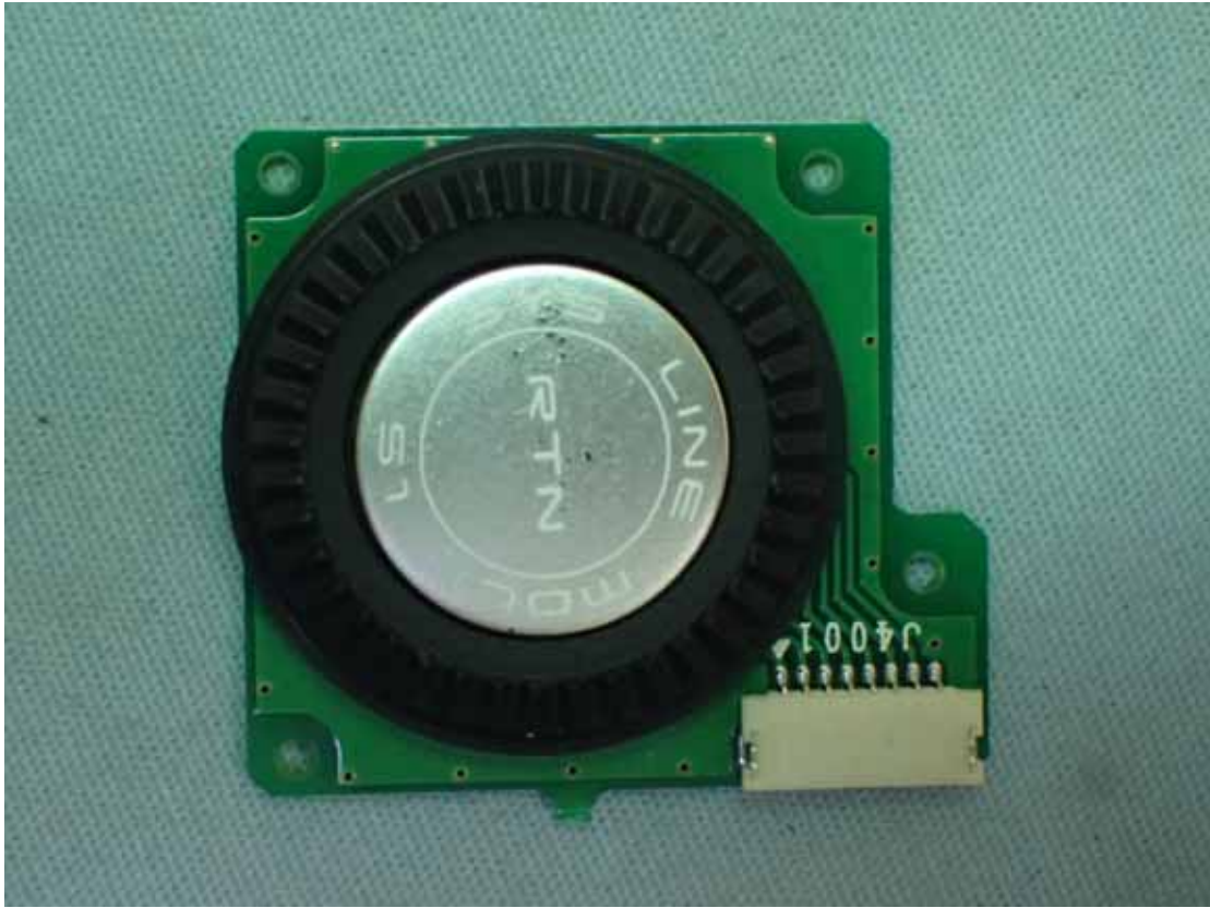
Figure 33 Internal View (Control Board, Front View)
