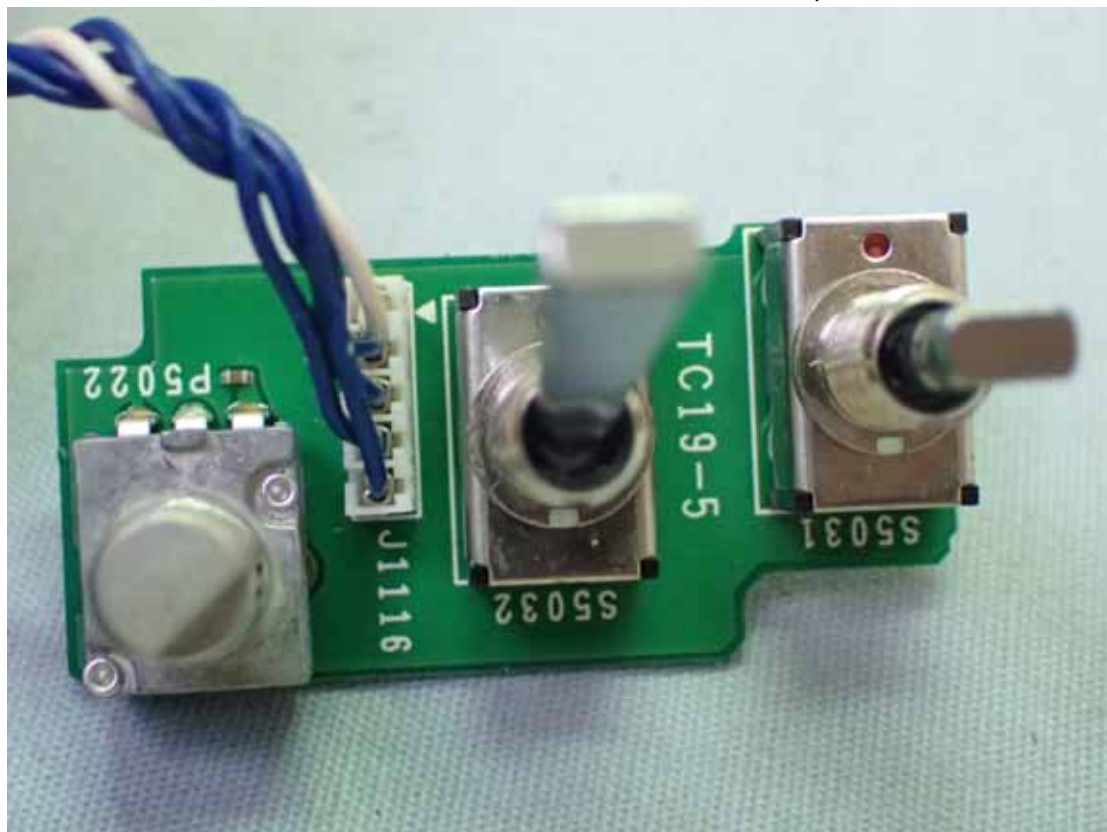
Figure 21 Internal View (Control Board, Front View)
