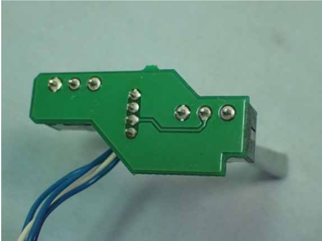
Figure 15 Internal View (Control Board, Back View)
