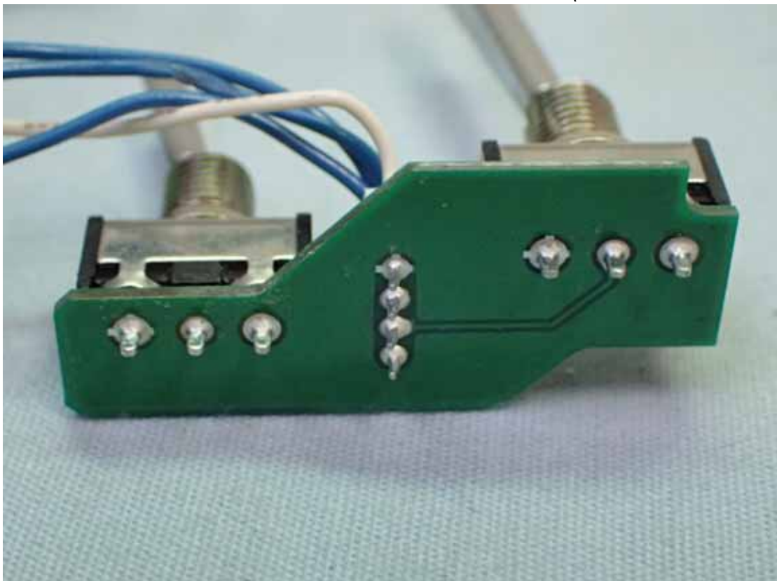
Figure 20 Internal View (Control Board, Back View)
