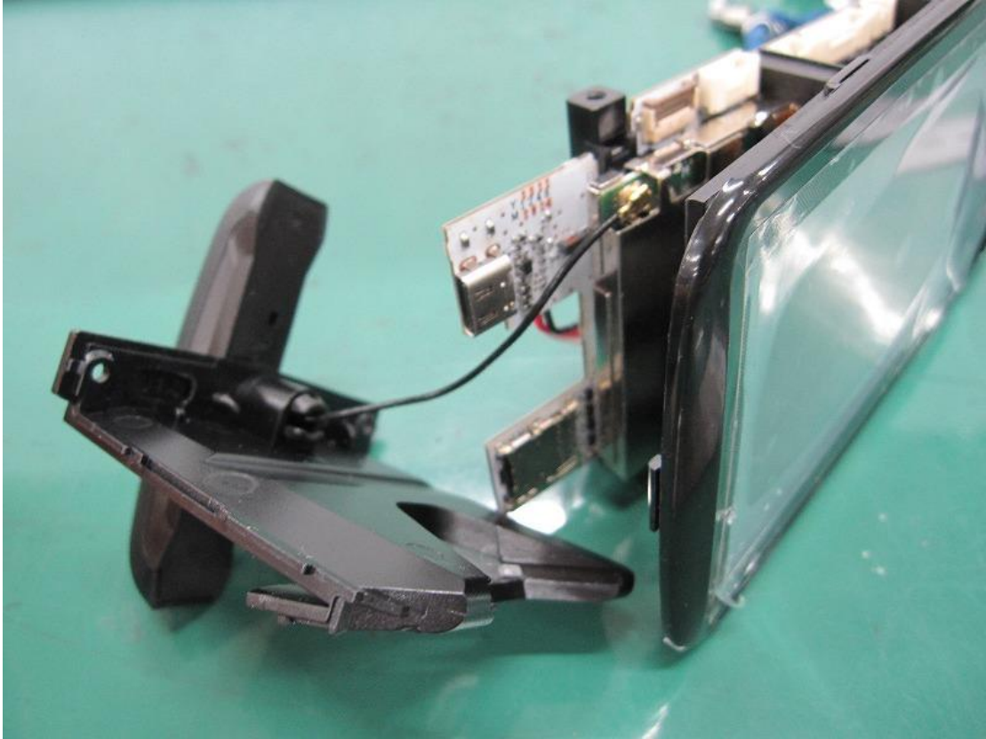
Figure 19 Internal View (Antenna Connect View)
