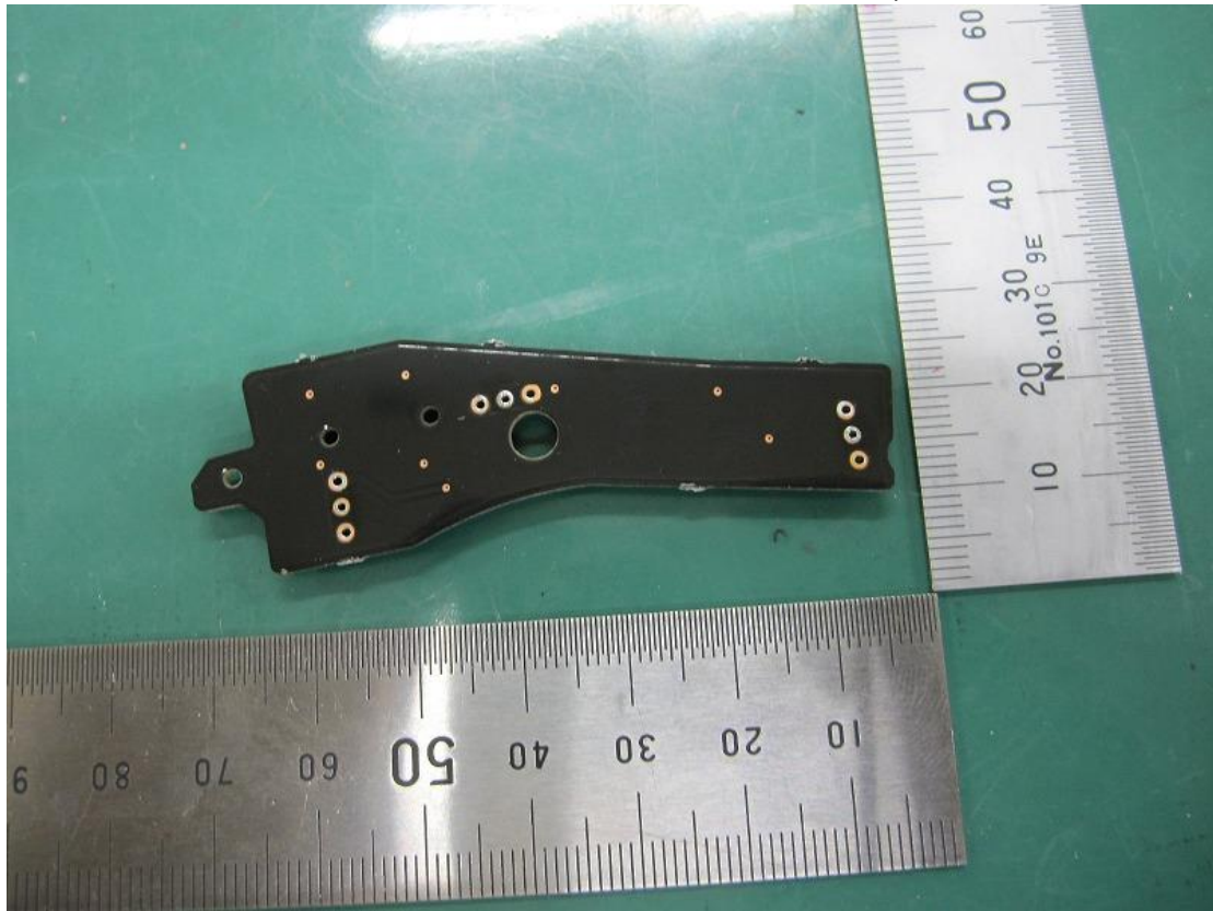
Figure 24 Internal View (Internal Board, Back View)
