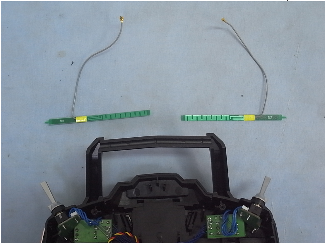
Figure 10 Internal View (Removed ANTs)
