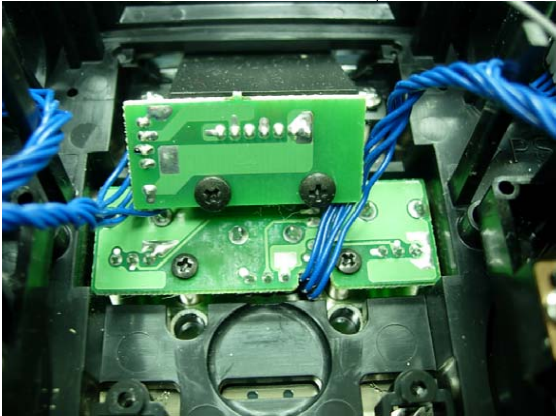
Figure 22 Internal View (TB24C-5 Board, Back View)
