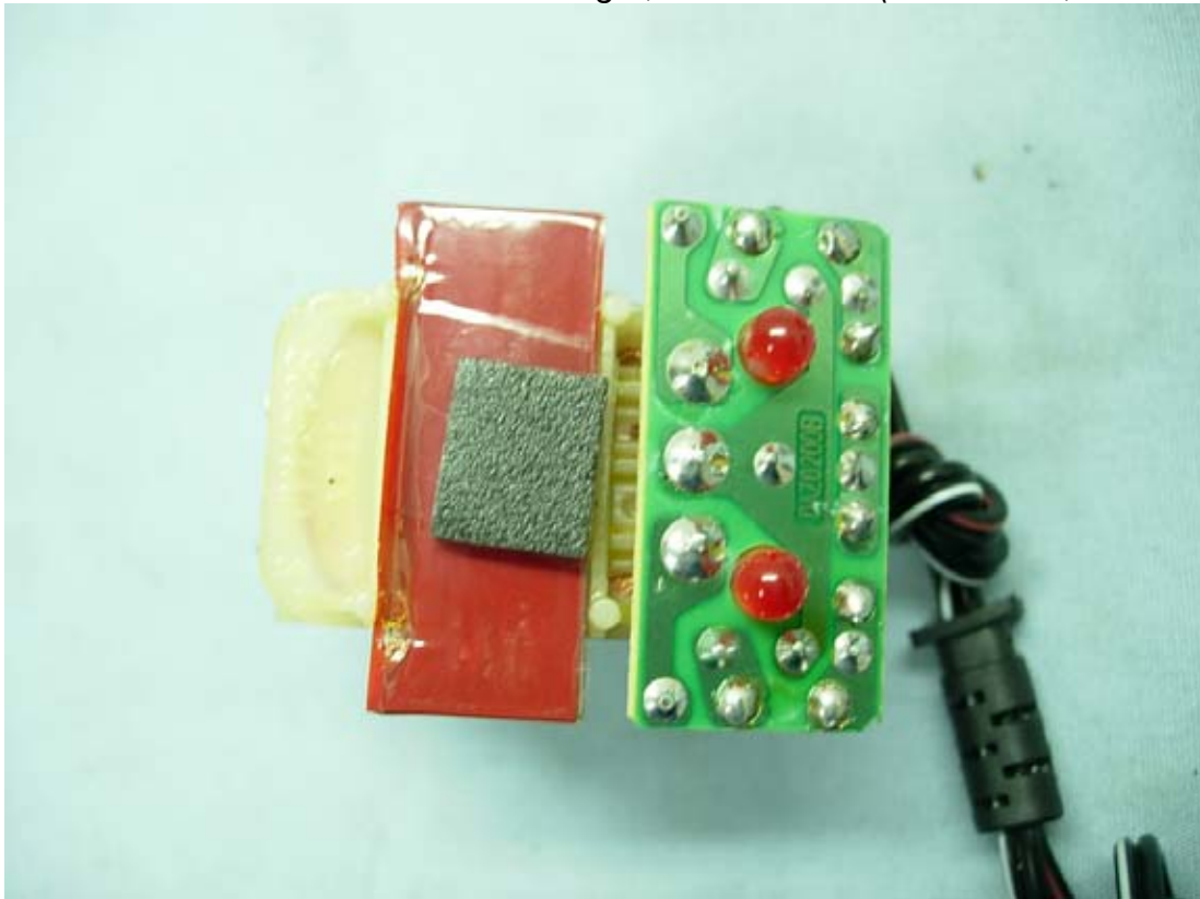
Figure 27 Ni-Cd Charger, Internal View (PCB Board, Back View)
