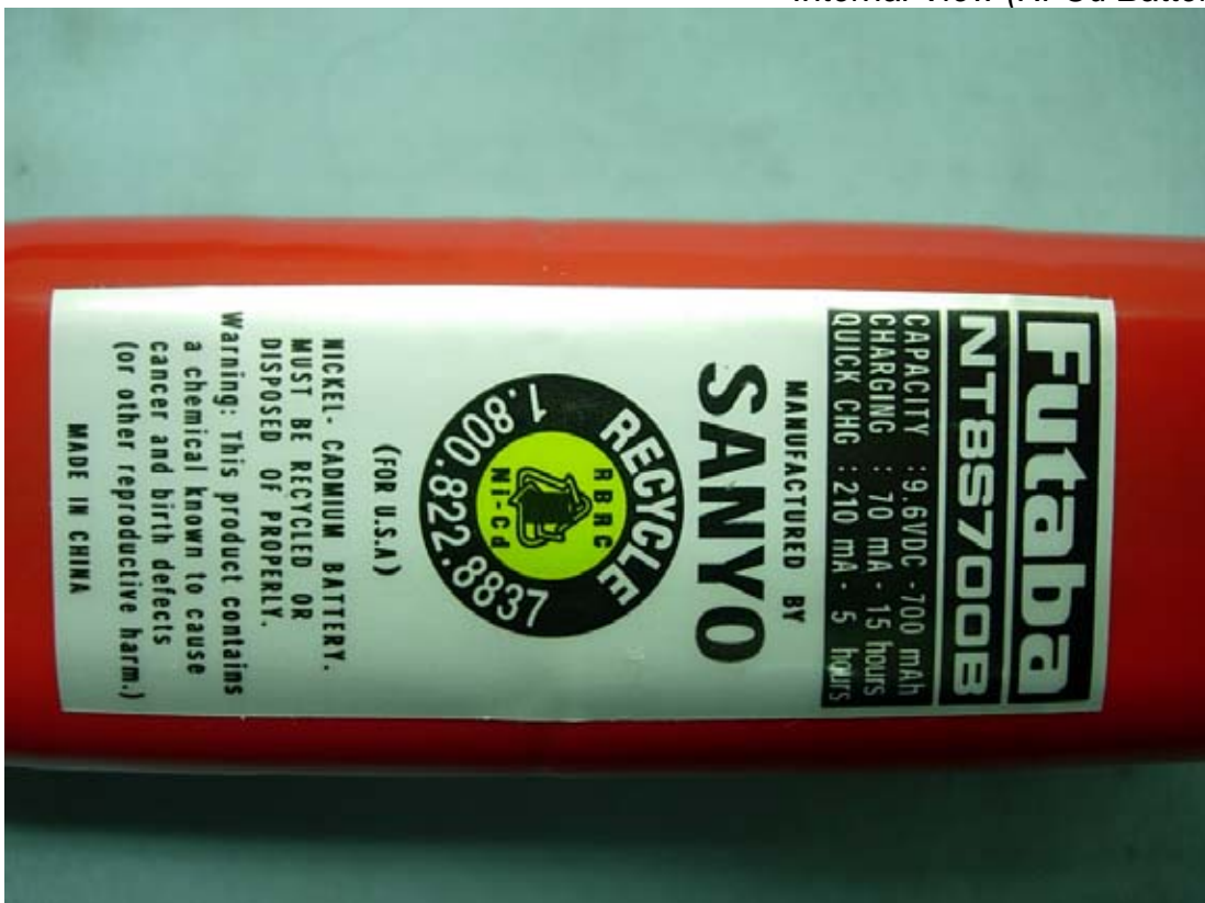
Figure 9 Internal View (Ni-Cd Battery Label)
