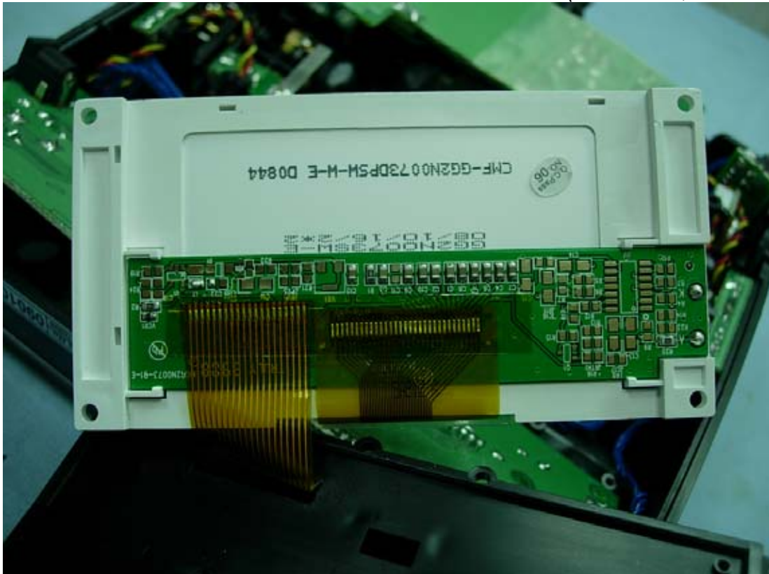
Figure 19 Internal View (LCD Panel, Back View)
