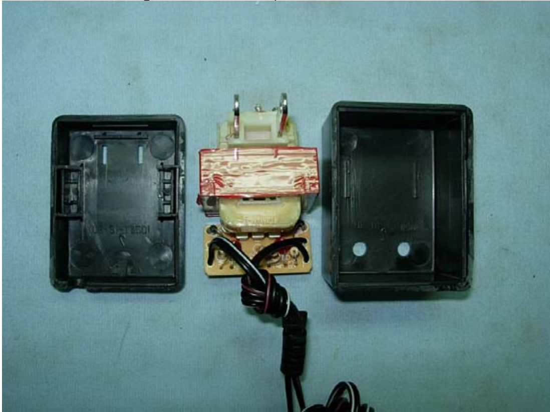
Figure 26 Ni-Cd Charger, Internal View (Removed Covers, PCB Board/Front View)
