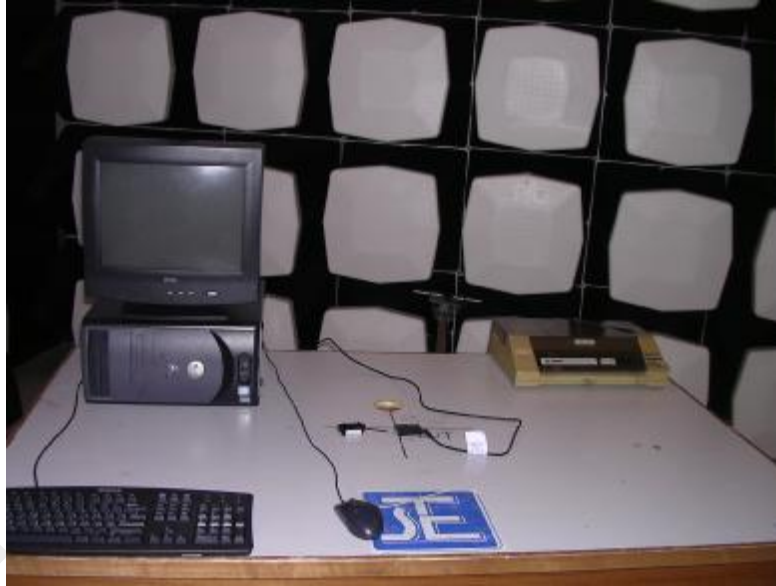
Measurement of Radiated Emission Test Set Up
