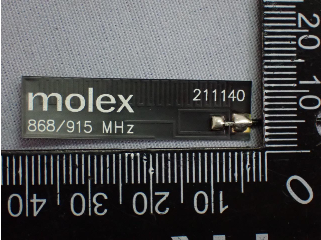
Figure 4 General Appearance (ANT A, Front View)
