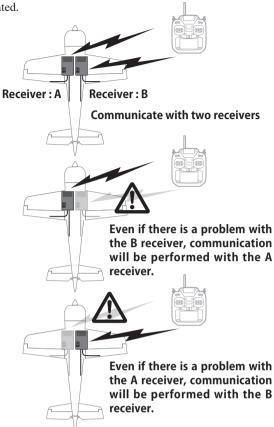
In Dual RX link mode, the SB2/RX port is for reception only, so use CH mode B, C, D, F, G, H mode for S.BUS output and S.BUS2 input/output.
