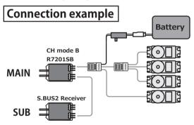
**Example of main R7201SB**: Use dual RX link mode of R7201SB. \*PWM3CH cannot be used.
