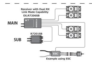
Example of sub R7201SB: Use dual RX link mode of R7206SB. \*Do not turn on the dual RX link mode of the R7201SB.
